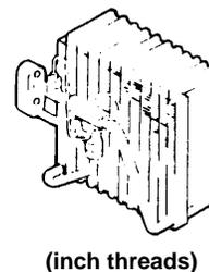
NOTE: The NSX R-134a evaporator has inch threads, therefore requiring an identification label. The Legend evaporator has metric threads with no label. Do not substitute R-12 parts for R-134a parts.
