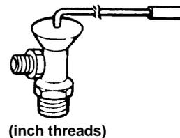
NOTE: The NSX R-134a expansion valve has inch threads, therefore requiring an identification label. The Legend expansion valve has metric threads with no label. Do not substitute R-12 parts for R-134a parts.
