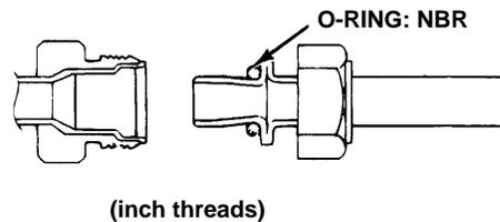
NOTE: The NSX R-134a piping has inch threads, therefore requiring an identification label. The Legend piping has metric threads with no label. Do not substitute R-12 parts for R-134a parts.
