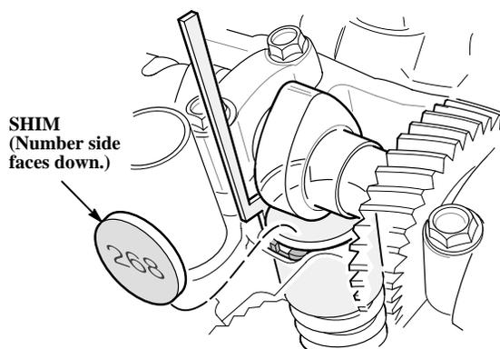
9. Release and remove the tool by turning the crankshaft clockwise again; keep turning it until the cam lobe again points away from the valve.
