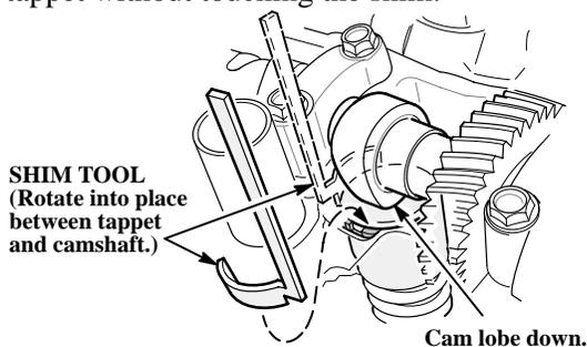
5. Slowly turn the crankshaft *counterclockwise* so that as the valve closes, the tool is caught between the camshaft and the tappet, holding the valve open slightly.
