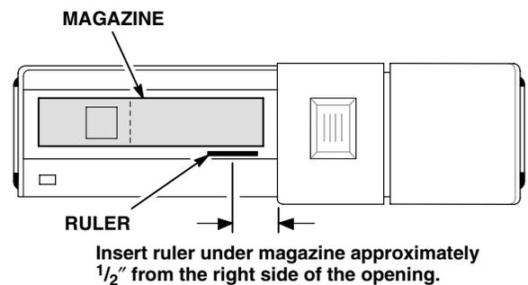
4. Push the ruler in until it presses against the eject lever at the back of the unit.
