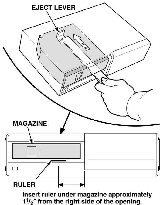
6. Push the ruler in until it presses against the eject lever at the back of the unit.
